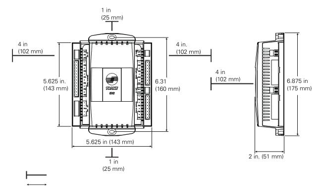
Figure 2. Metal-cover model dimensions and clearances
